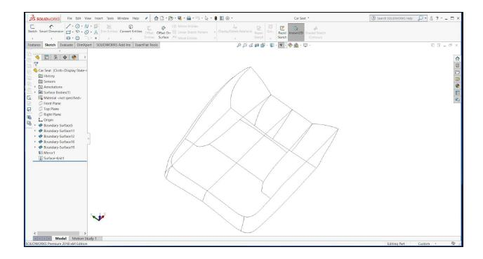
An STO file may or may not be provided with seam lines drawn directly onto the 3D Model using line entities or faces split where seams are intended. To handle both cases, 3D sketch lines are inserted into the 3D model, outlining where splits must occur. From that information the manufacturing team can edit the 3D solid into the separate 3D pieces.
