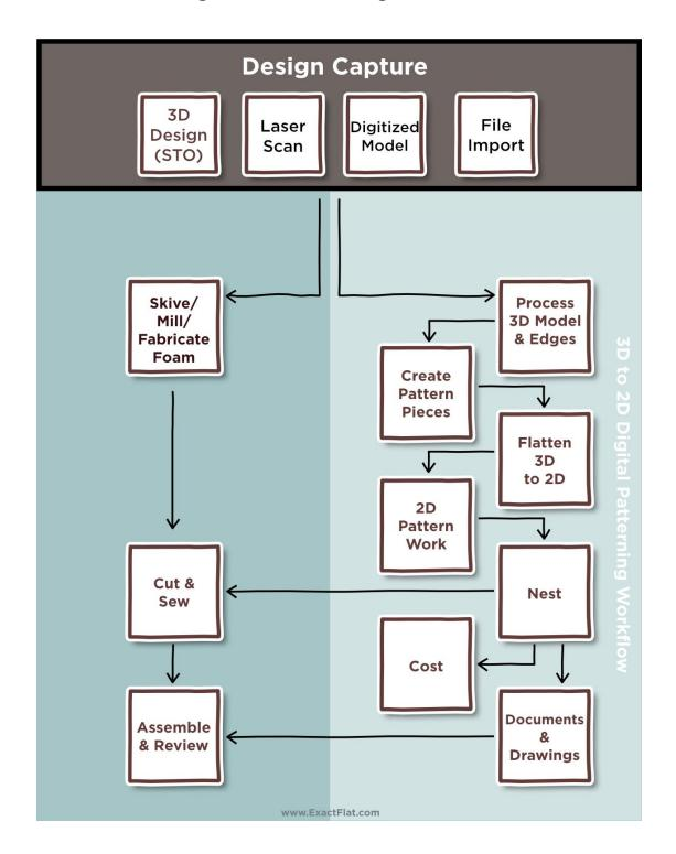
The chart above uses the example steps for automotive seating trim, however, the 3D to 2D digital patterning workflow, applies to all transportation interior soft goods.
