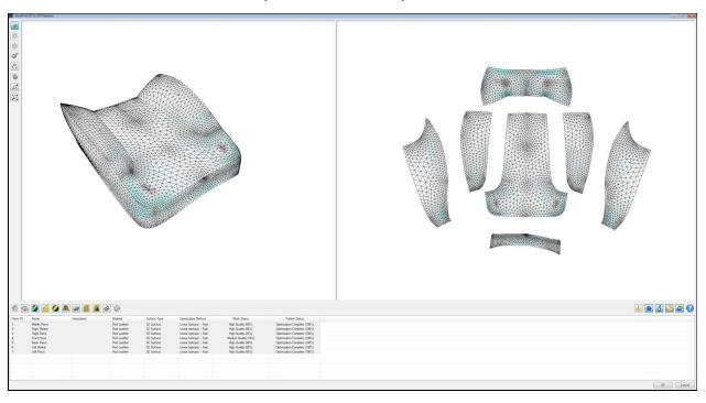
The next step is to enter the pattern environment in order to flatten the design. After selecting the patterning menu, ExactFlat generates a flat pattern layout for each material in the design. Strain and sag displays are mapped on both the 3D model and 2D pattern pieces. This information is then used to help determine if edits, such has relief cuts are needed to ensure
