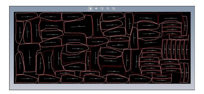
As with all of the digital patterning features, Nesting integrates directly with the 3D design and 2D patterning environments. Users simply
